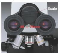
adjustment and diopter setting. High eyepoint design eyepieces with F.N. 20 can be used comfortably without removing eyeglasses.
